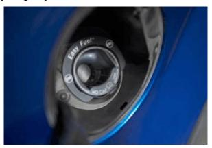
**NOTE:** Stant also makes an aftermarket Instant-Fill or NASCAR<sup>TM</sup> fuel cap available for most makes and models. This type of gas cap is also acceptable but should be suspect if EVAP codes are present.
