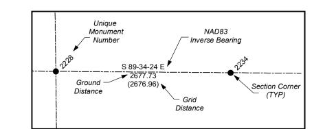
ALL BEARINGS AND DISTANCES SHOWN ARE BASED ON THE UTAH COORDINATE SYSTEM, 1983 CENTRAL ZONE.
